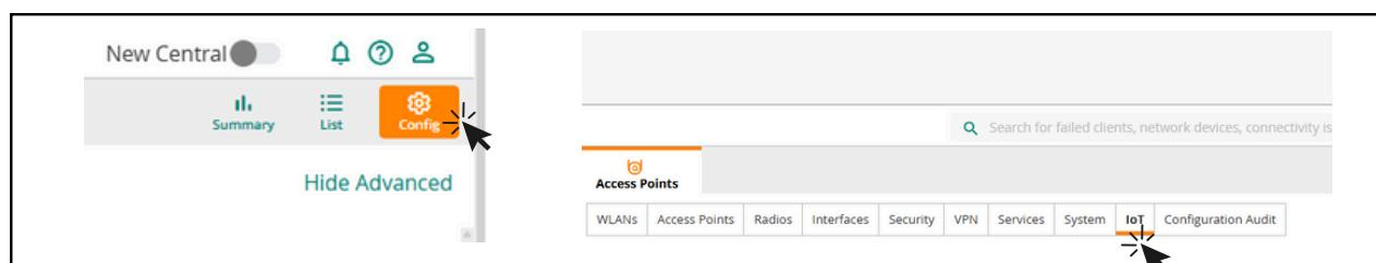
2.1.3 Create a new IoT Radio Profile using the '+' sign and **set the 'Radio Mode' to BLE (1)**.
