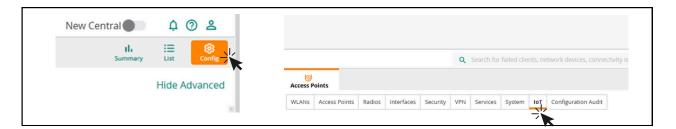
Create a new IoT Radio Profile using the '+' sign and set the 'Radio Mode' to BLE (1).
