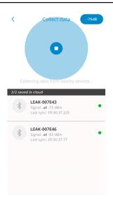
After successfully collecting data, the sensor will be moved to the bottom of the list, categorized under 'Saved in Cloud.' There, you will see only a green light and a timestamp indicating the last synchronization of data, referred to as 'Last sync'.
