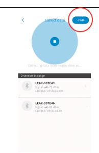
Choose the desired Bluetooth range by clicking on the blue icon in the upper-right corner. If you are close to sensors, we recommend starting from -65 dBm. Wait until the data from the detected sensors are collected, then increase the Bluetooth range incrementally. This approach allows you to collect data from the nearest sensors first, ensuring better and faster data retrieval.
